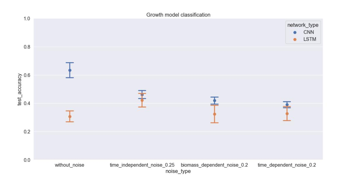
**Above.** Classification results for LSTM and CNN models dealing with different sources of noise. Models were trained with and without additional features from DE-based models. The CNN with additional features outperformed the LSTM in the case of noiseless data. Noise considerably affects correct classification by ML (courtesy of Yingjie Shao).
