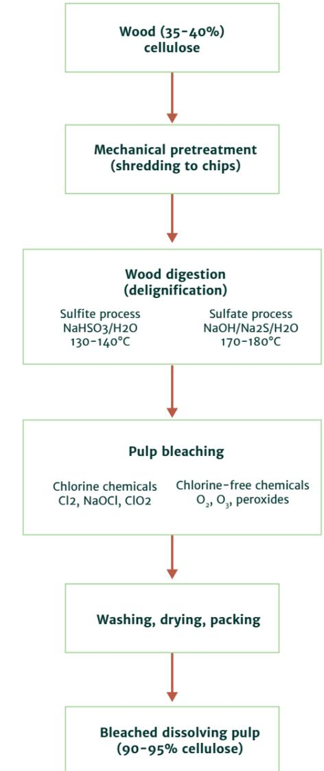
**Figure 2.4** Key stages in the manufacture of viscose and lyocell fibres
