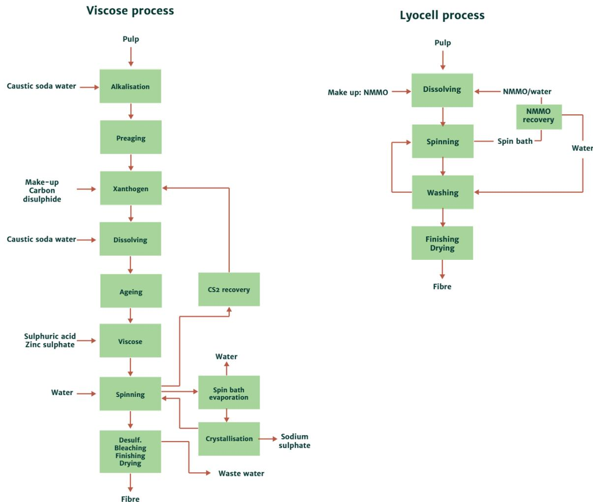
**Figure 2.5:** Production route of biomass to bio-based synthetic fibres
