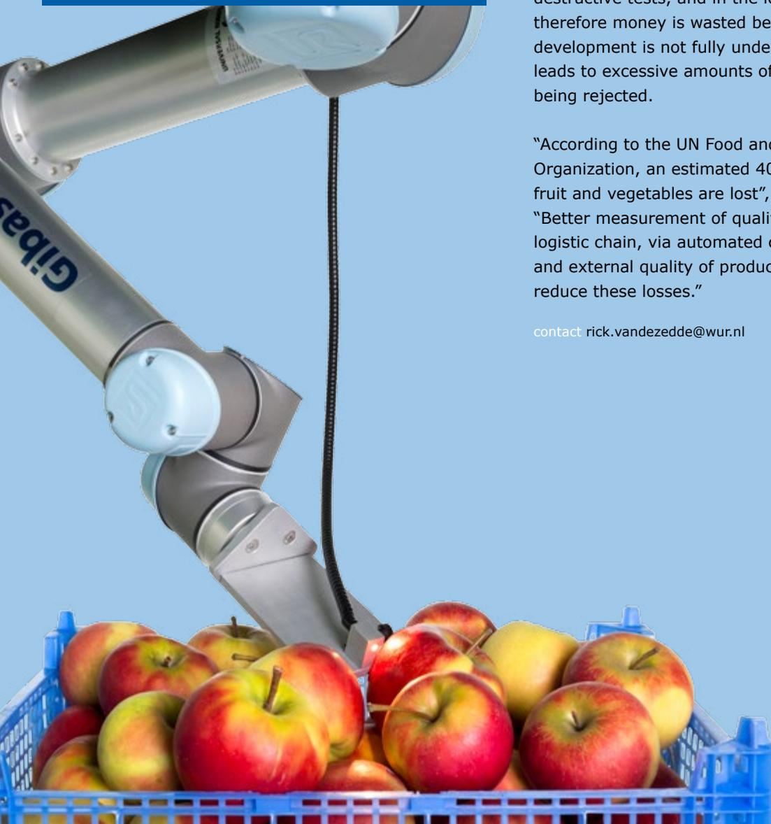
The robot, developed as part of the GreenCHAINge project and based on the technology of high-speed sorting systems, is able to test a variety of external and internal quality factors, non-invasively, such as dry-matter content, firmness and sweetness. Although it mimics a human quality-expert, it combines more-objective and reliable data with much higher capacity.
